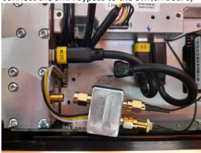
3. connect the Switch Board to the DCM.
