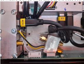
2. connect the SMA bypass to the Switch Board,
