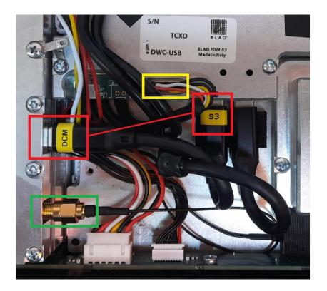
Connect the USB-C cable respecting the direction, as stated by the cable marks.
