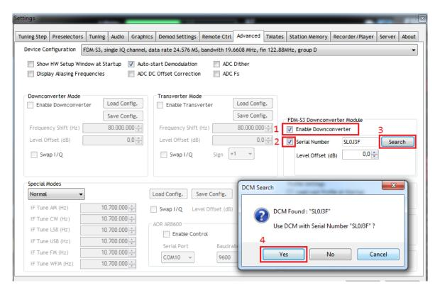
If the Downconverter is working correctly (above 108MHz), "DCM" is displayed to the right of the S3 serial number, like this:
