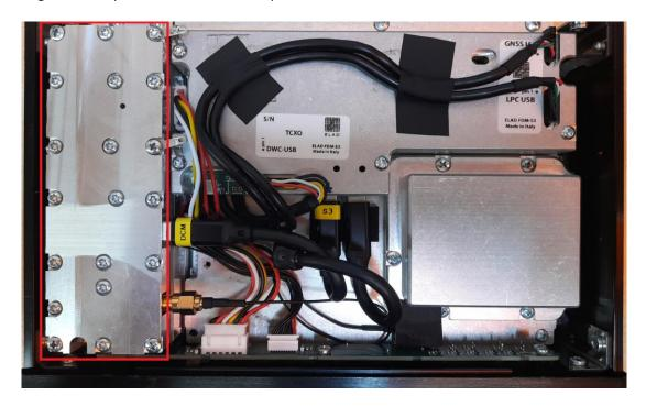
The Downconverter must be fixed to the lower panel by means of 4 screws and the 2 tab washers must also be fixed to the field of the RCMM (Reference Clock Manager Module):
