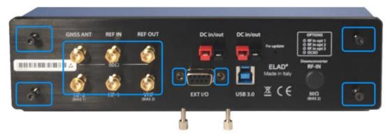
Remove the top cover. Once the screws have been loosened, move the rear panel slightly outwards in order to remove the top cover. Attention, the bottom cover will also be free from the frame.
